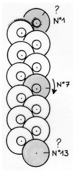
The clock shown is found in the Dynamikum Science museum in Pirmasens, Germany. It is made up of thirteen identical large cogwheels. Each large cogwheel contains a pinion with the same axis. A pinion has exactly seven times fewer teeth than the large cogwheel. Each pinion drives the large cogwheel beneath it.
